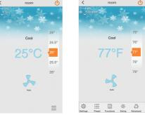
3. Fan Speed: It used for setting fan speed. Under cooling or heating mode, if the noise-customized function is turned on, adjust the fan speed and then the noise-customized function will be turned off automatically. Please refer to the part of remote
