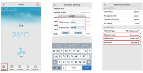
7. After modifying name and password, click it to return and there will be a prompt box, and then clock "OK" to finish the modification. Meanwhile, the software will turn back to interface of "Air-Conditioner" and the AC list will be gone.
